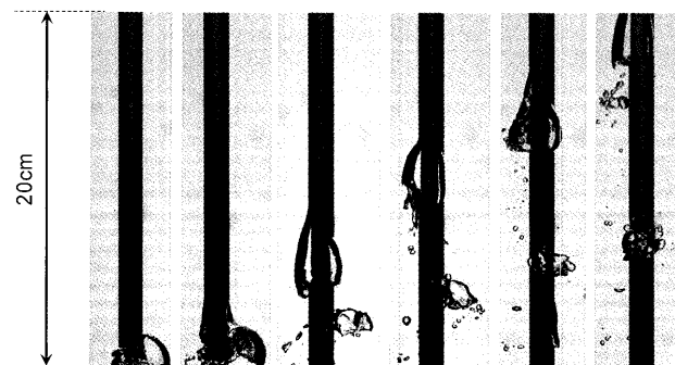
Fig. 12. Rising bubble ( \theta=144^\circ , D=1.6 cm, V_B=15\text{ cm}^3 ). (Photographs were taken successively at a time span of 0.05 s. Time elapsed from left to right.)
