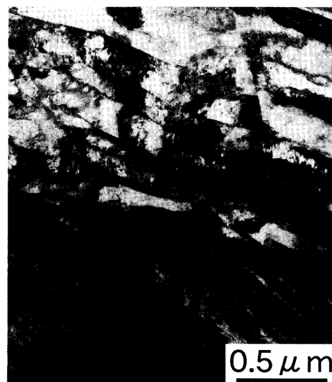
Fig. 8. Enlarged bright-field image around the border between T-M lamellae and shear band.
