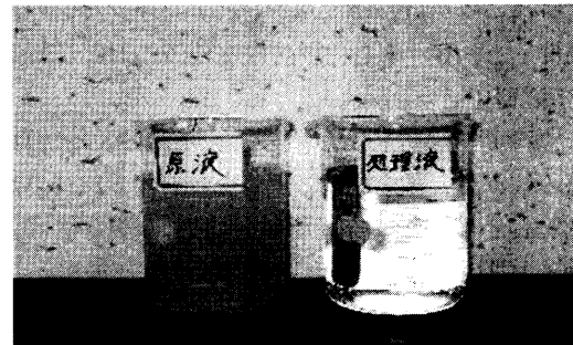
Fig. 15. Photograph of wastewater before and after treatment by gas-liquid two-phase swirling jet and ozone (left: original, right: treated).
