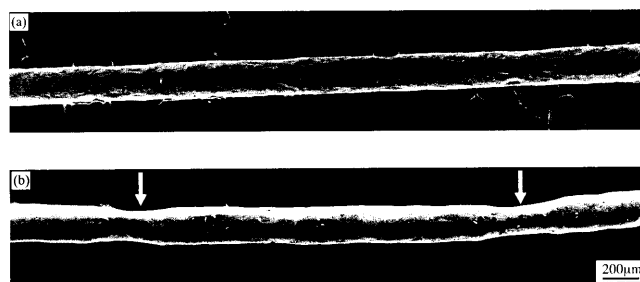
Fig. 8. Scanning electron micrographs of SUS316 ( \phi 0.2 mm) wires tensile-deformed by fracture. The D/d is controlled to be 8.0 (a) and 2.2 (b), respectively.
