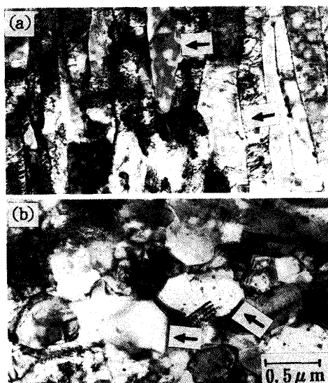
Fig. 6. Transmission electron micrographs for A4 steel with reversion treatment of 600^{\circ}\text{C} \times 20\text{h} after (a) As quenching and (b) 50% cold rolling.
