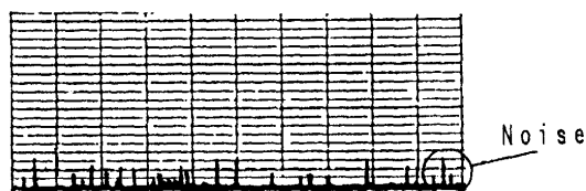
(a) Signal chart of ECT used conventional sleeve.
