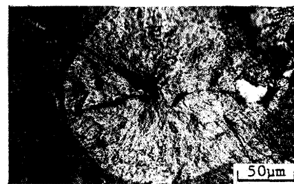
HV=675, \sigma=980\text{MPa} , N_f=6.91 \times 10^6 , \sqrt{\text{area}}=9.8\mu\text{m} Distance from surface=93 \mu\text{m} Chemical composition: Ti-Mn-C-S
