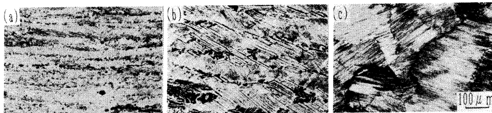
Fig. 6. Microstructures of Ti-47.3at%Al deformed in the \alpha+\gamma phase field, (a)1573K, (b)1598K and (c)1623K, and cooled at 50K/s.
