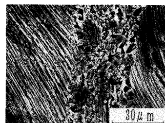
Fig. 9. SEM image of Ti-44.4at%Al deformed at 1473K and cooled at 50K/s.
