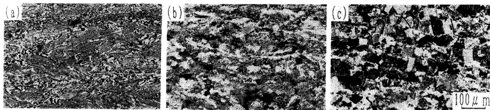
Fig. 7. Microstructures of (a)Ti-44.4at%Al, (b)Ti-47.3at%Al and (c)Ti-48.4at%Al deformed at 1473K and cooled at 0.1K/s.
