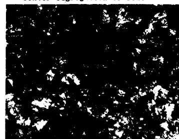
Phot.2 Micro Structure of longitudinal cross section of hot coil
