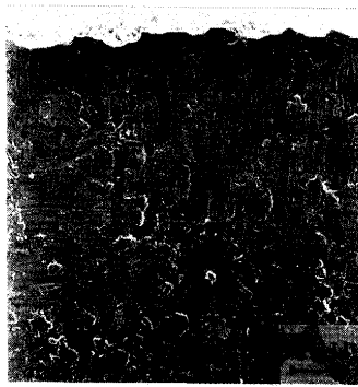
Fig. 13. Fretted surface in LiCl-CH 3 OH (STA). \sigma_a = 130\text{MPa} , P = 50\text{MPa} , N_f = 2.63 \times 10^6 cycles
