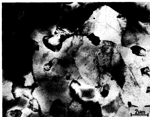
Fig. 11. Transmission electron micrograph of Hastelloy X creep-tested for 15 h at 850°C and 78.5 MPa (Rupture life : 40 h).
