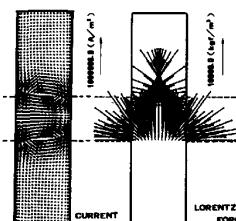
Fig. 3 Calculated current density and Lorentz force.
