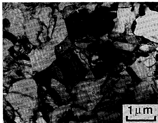
Photo. 9. TEM microstructure of fine recrystallized grains formed from the reversed austenite in 14Cr-11Ni steel annealed at 923 K for 10 s after 96% cold rolling.
