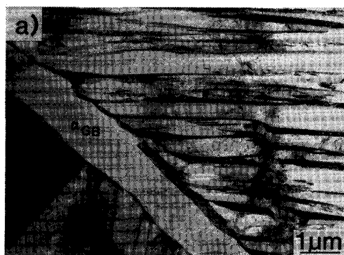
a) Grain boundary \alpha ( \alpha GB) and fine lamellar structure (F. L.) shown in Photo. 1 b) The inner area of prior \beta grain Photo. 4. TEM micrographs of Ti-6Al-4V cooled from 1050°C at the cooling rate of 10°C/s to room temperature.
