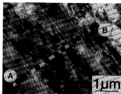
Fig. 2. EDS analysis for the same specimen as shown in Photo. 3. Analyzed points are along the line from A to B in the photo. \overline{C(Al)} , \overline{C(V)} , \overline{C(Fe)} represent the nominal compositions of Al, V, Fe respectively.
