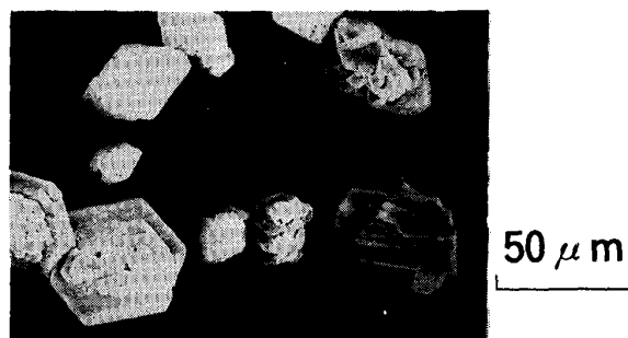
Photo. 2. Phosphophyllite crystals precipitated from the synthetic solution.
