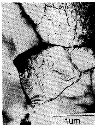
Photo. 5. TEM micrograph showing the fine ferrite grains obtained by stress controlled tensile testing of steel SCM418 shown in Fig. 7 (a).
