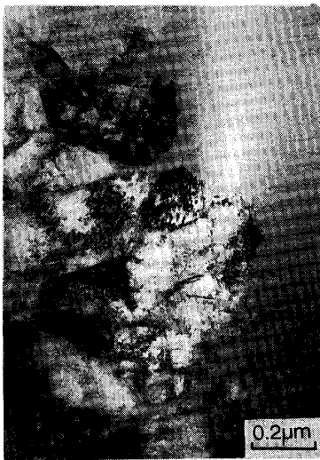
Photo. 4. Microstructure of laser treated layer after wear test (Test B).
