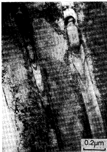
Photo. 5. Microstructure of laser non-treated sample after wear test (Test B).
