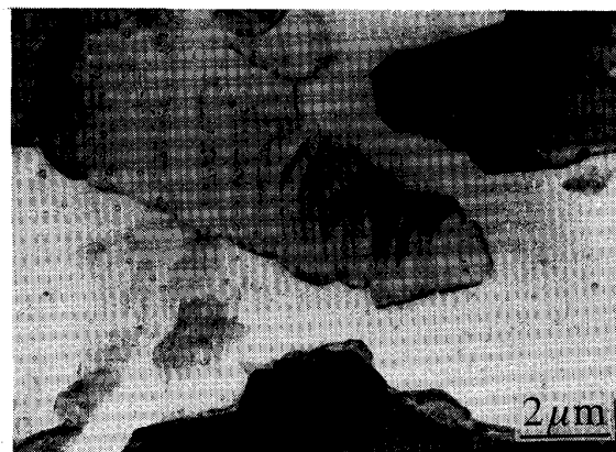
Photo. 6. Graphite morphology formed on the surface of steel sheet annealed at 700°C for 5 h in vacuum.
