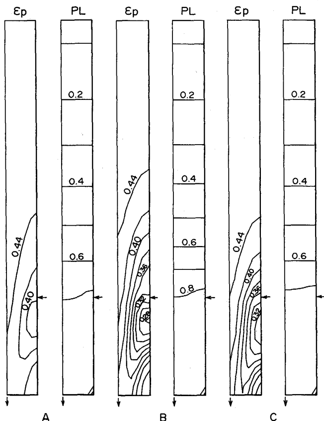
Fig. 13. Void ratio of packed bed and pressure level of the SC pilot plant during the connection operation 3) calculated by the two dimensional mathematical simulation model.
