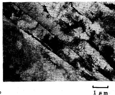
Photo.1 Transmission electron micrograph showing microstructure at mid-thickness of Al-Ti-B steel plate.
