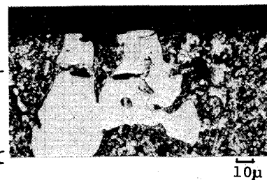
photo.1. Microscopic picture of worn surface. (carbide distance--narrow)
