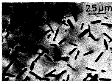
6362 ruptured after 718h
