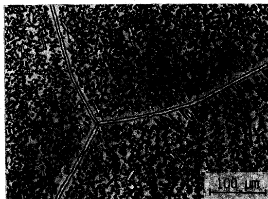
Photo. 1. Optical micrograph of \alpha - \gamma two phase structure before the aging tests.
