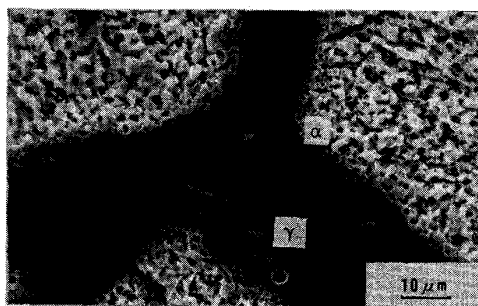
Fig. 6 A SEM image after oxalic acid etching of a water cooled specimen. PT=1350°C
