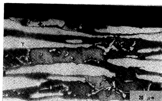
Fig.8 A microstructure of a cracked specimen of the girth weld joint. (100°C, P H 2 S =0.8kg/cm 2 , 5%NaCl)
