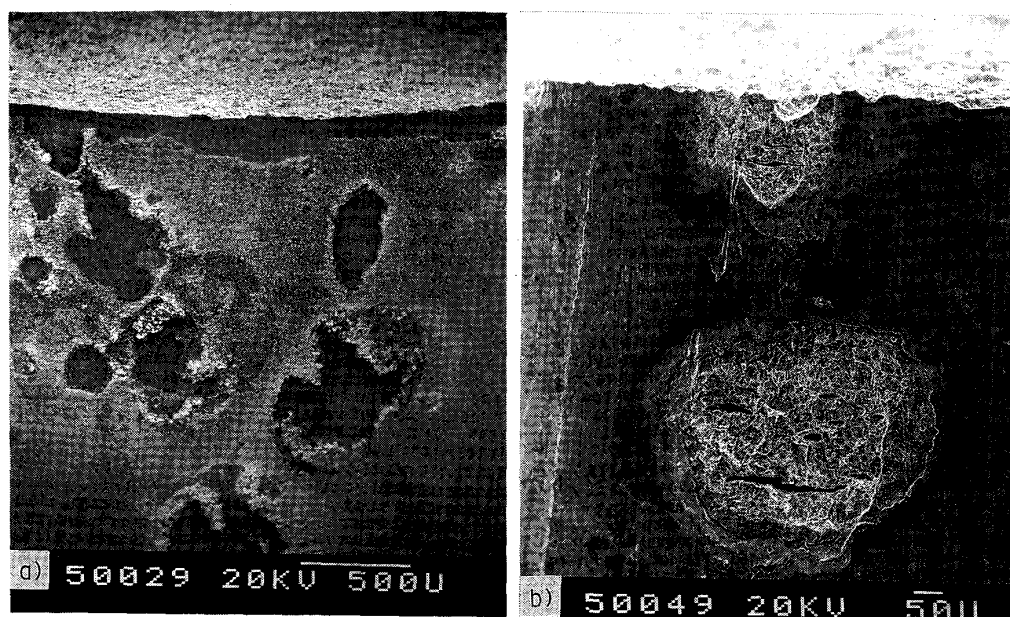
a) Sea water at constant flow rate ( \Delta\sigma_a=12.5 \text{ kgf/mm}^2 , N_f=4.3 \times 10^6 ) b) Sea water or air for every 1 min ( \Delta\sigma_a=9.7 \text{ kgf/mm}^2 , N_f=4.5 \times 10^6 )
