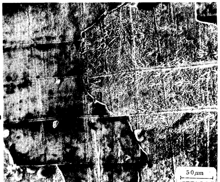
Photo. 2. Scanning electron micrographs showing the oxide cracks on the specimen surface after low cycle fatigue failure.
