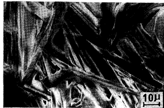
Photo. 8. SEM image of calcium ferrite formed on pseudo-ore containing no \text{SiO}_2 and no \text{Al}_2\text{O}_3 .
