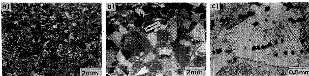
a) Quenched at 1470°C ( T_\gamma + 5^\circ\text{C} ) b) Quenched at 1460°C ( T_\gamma - 5^\circ\text{C} ) c) Higher magnification of the grain indicated by an arrow in b), showing \gamma grain boundary Echant: a), b); 2% nital and c); Picric acid 0.15% C-1.48% Mn steel cooled at a rate of 0.1^\circ\text{C s}^{-1}
