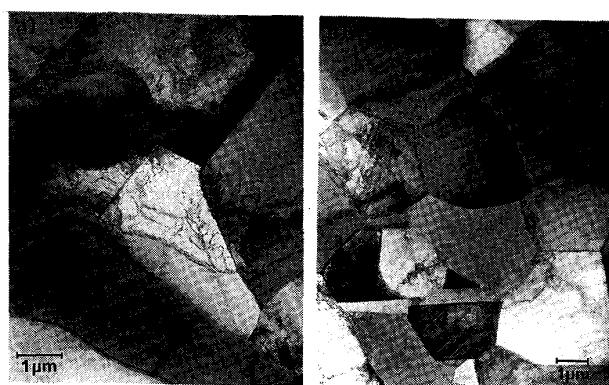
Photo. 8. TEM micrographs of steel D2; priorly cold-rolled and deformed to 100% elongation at 900°C at \dot{\epsilon}=4.16 \times 10^{-3} \text{ s}^{-1} .
