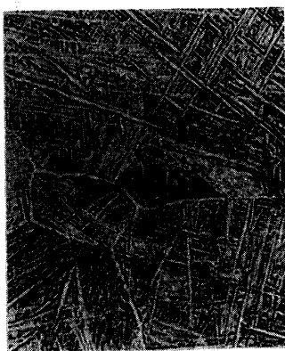
(a) \beta Extruded, Air Cooled and Annealed
