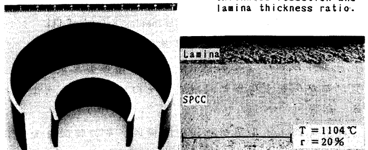
Photo 2 Bending of the manufactured metal-metal composite cladding sheet and its internal structure. (Mother sheet: SPCC, Lamina: Cast iron)
