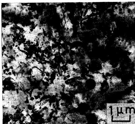
Fig.2 Microstructure observed on the cross section of an as-extruded Al-8Fe-2Mo alloy.
