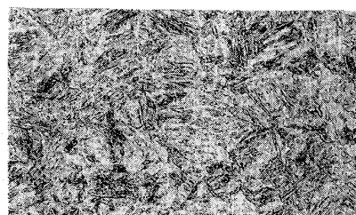
Photo.1 Micro structure (40mm t, 1/4 t)
