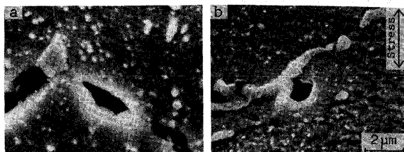
a) Creep t=1500h(t/tr=0.8) b) Creep + sintering + creep t=1450h (Point B in Fig.2)
