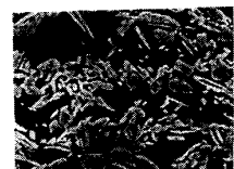
Photo 1 Microstructure of R.Q. type 980 MPa grade steel sheet.
