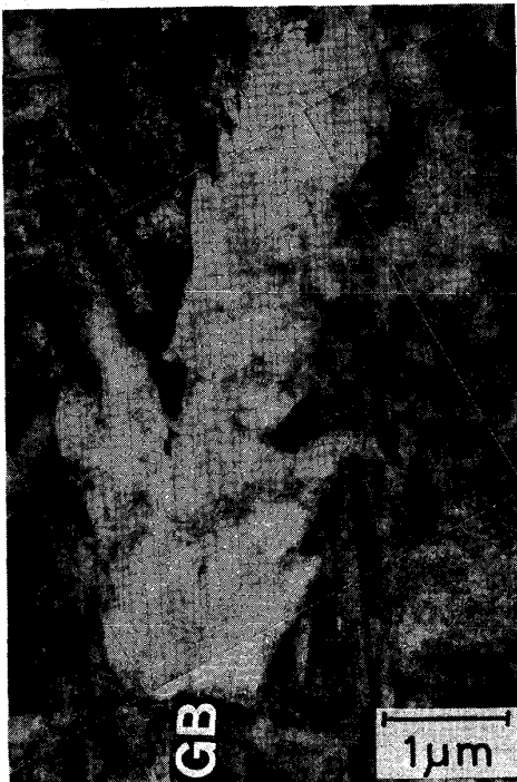
Fig.1 Proeutectoid ferrite formed at the austenite grain boundary
