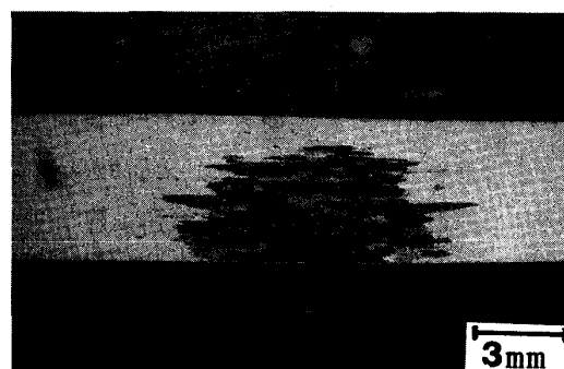
Photo. 2. Partial grain growth by the strain(&lt;30%) annealing
