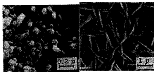
Fig.1 SEM micrographs of various Zn-polymer composite coatings
