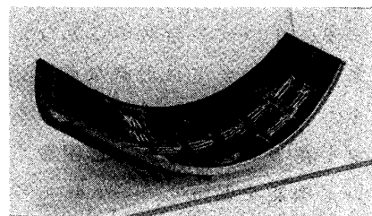
Photo.1 Appearance of full-sized model for cold-pressed tank corner of LPG carrier
