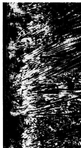
Fig.2 Morphology of columnar dendrites in the position of ripple mark. (x11.3)
