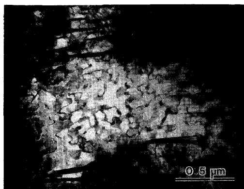
Photo. 3. Domain structure of \text{ZrO}_2 -4 mol% \text{Y}_2\text{O}_3 alloy. The micrograph was taken by a 112 reflection, which is forbidden for cubic fluorite structure 56) .
