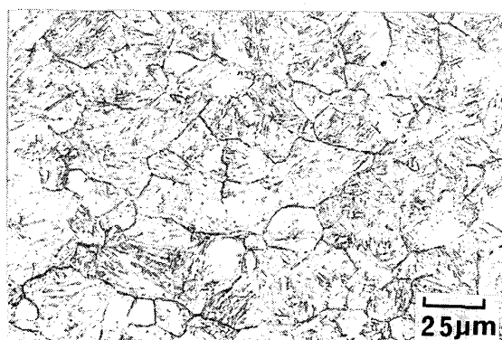
Photo. 6. Microstructure of steel J8 with embrittling treatment revealed by grain boundary etchant.
