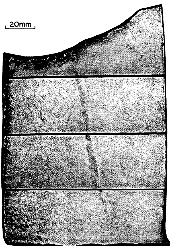
Photo. 1. "A" segregation reproduced in a 14 kg ingot containing 0.13%Nb and 0.09%Ta.
