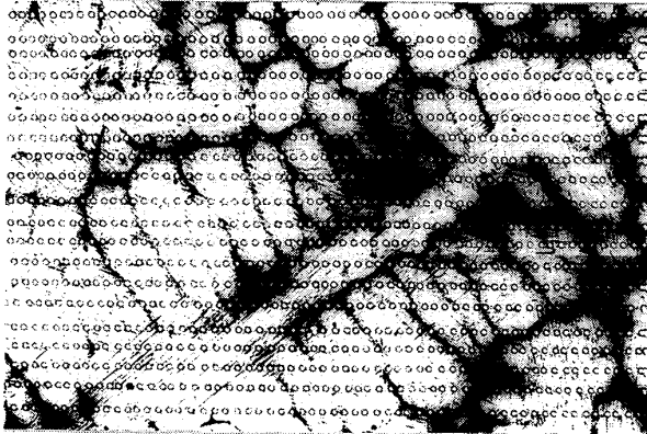
Photo. 5. Solidification structure of a commercial carbon steel specimen containing 0.28\text{ wt}\%\text{C} quenched at 1486^{\circ}\text{C} during the process of continuous cooling. White circles indicate the positions of scanning electron beam of EPMA. ( \times 100 )
