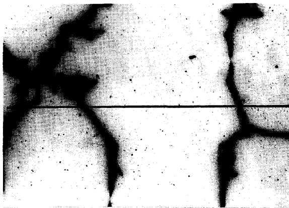
Photo. 2. Solidification structure of a Fe-0.29 wt%C alloy specimen which was cooled down to 1440°C at a cooling rate of 0.15°C/s after keeping for 1 h at 1498°C and was quenched at that temperature. Solid line in the photograph shows the scanning path of EPMA. ( \times 75 )
