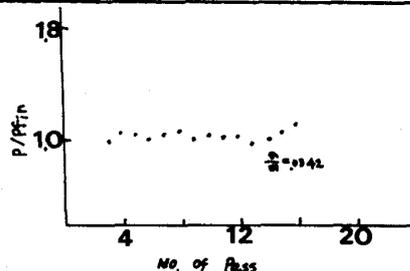
Fig.1. Ratio of measured (P) and calculated rolling load ( $P_{fin}$ )
