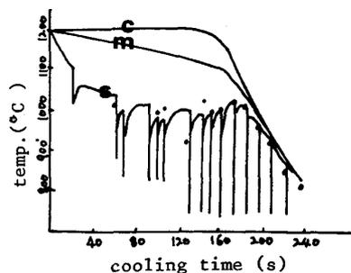
Fig.2. Comparison between calculated and measured temperature. C:center temp., m:mean temp., S:surface temp., • : measured surface temp.
