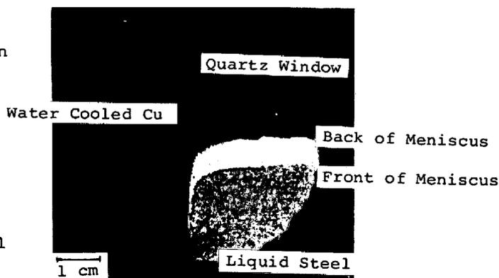
Fig. 1 Shape of ascending steel meniscus (Conditions; air atmosphere, static water-cooled Cu mold)
