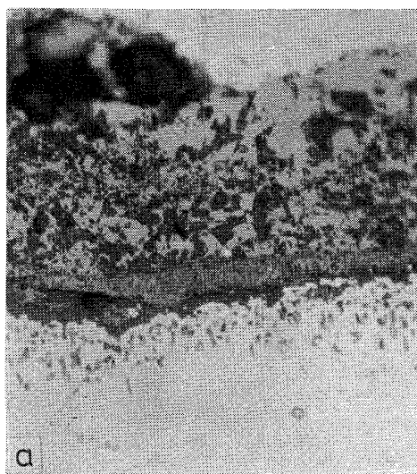
Photo. 1. Microstructures of section of scales formed on M (a) and MR2 (b) alloys after 10 cycles in cyclic oxidation heating for 25h at 1200^{\circ}\text{C} -cooling in air.
