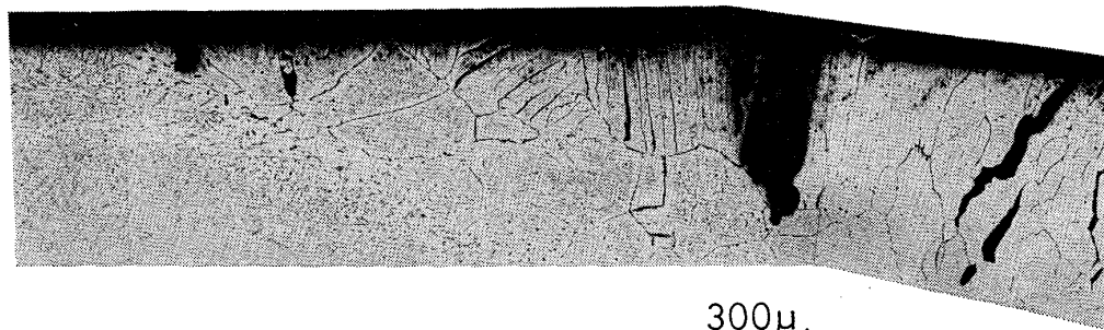
Photo. 3. Intergranular corrosion of 25Cr-6Ni-0.4Cu-2Mo-low N welded joint without a filler metal in Mod. Strauss test.
