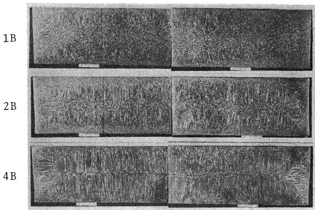
Photo. 8. Macrostructures of continuously cast slabs with vibration.
