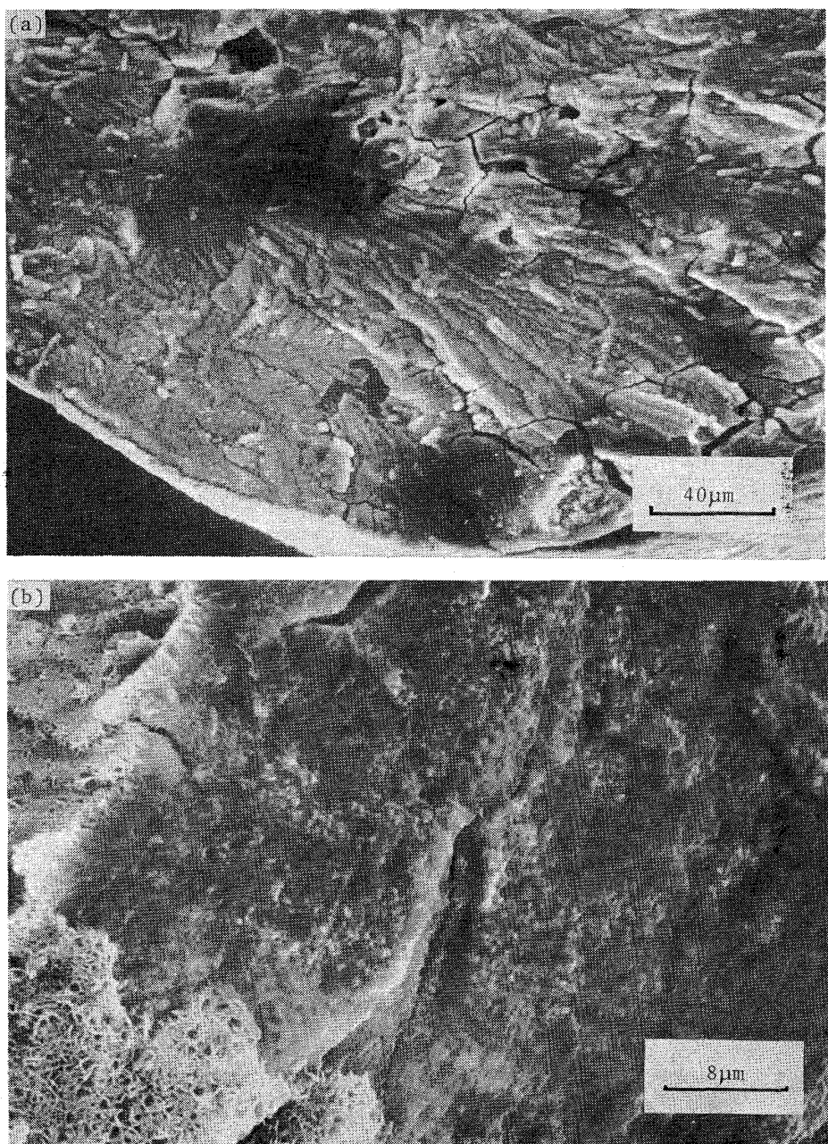
(a) 45% \text{MgCl}_2 , 154°C, 5 kg/mm 2 , t=243 min (b) 45% \text{MgCl}_2 , 154°C, 5 kg/mm 2 , t=243 min
